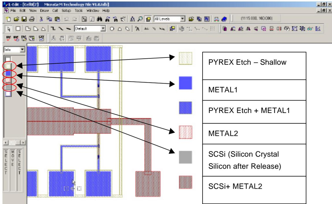
**Figure 2-5: Layers in the Micragem Technology File**
