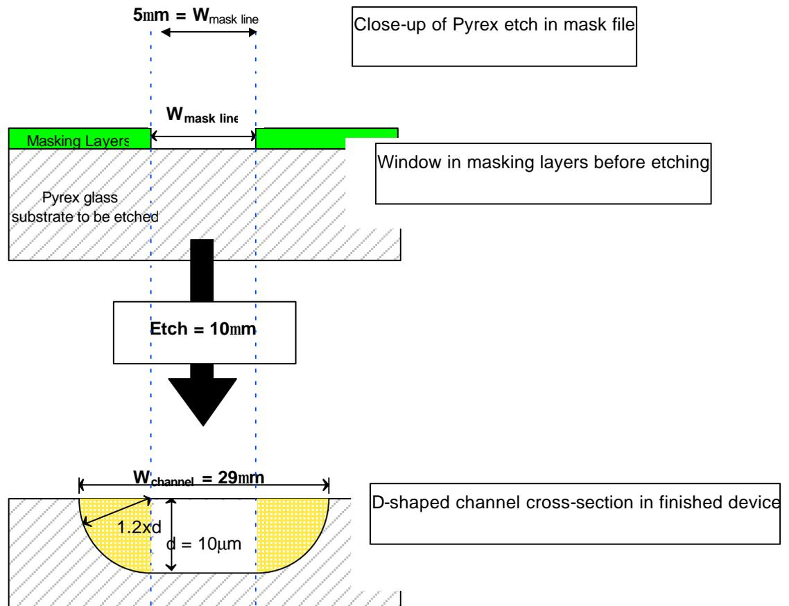
**Figure 3-2: Appearance of Features Before and After Isotropic Etching**
