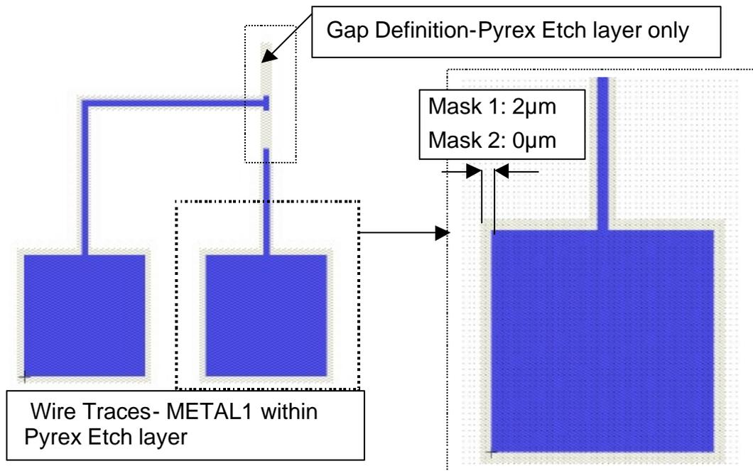
**Figure 3-4: METAL1 Features Appear within Pyrex Etch Features**
