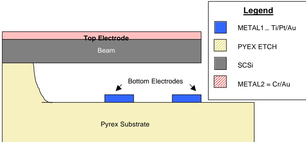
Figure 2-1: Side View of Cantilever Beam Designed with Micragem
