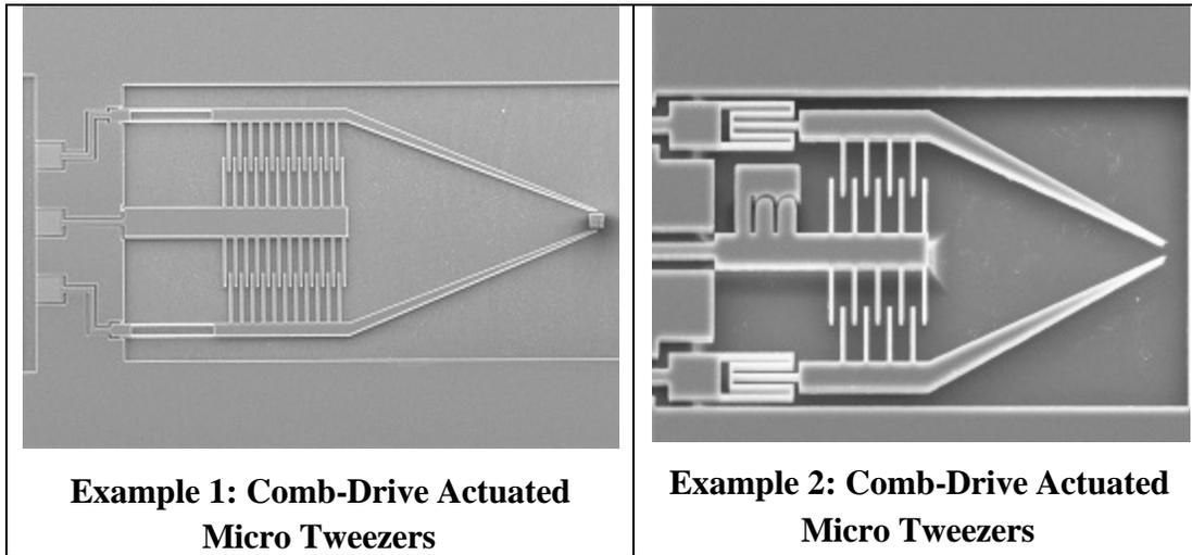
**Figure 6-1: Comb-Drive Actuated Micro Tweezers**
