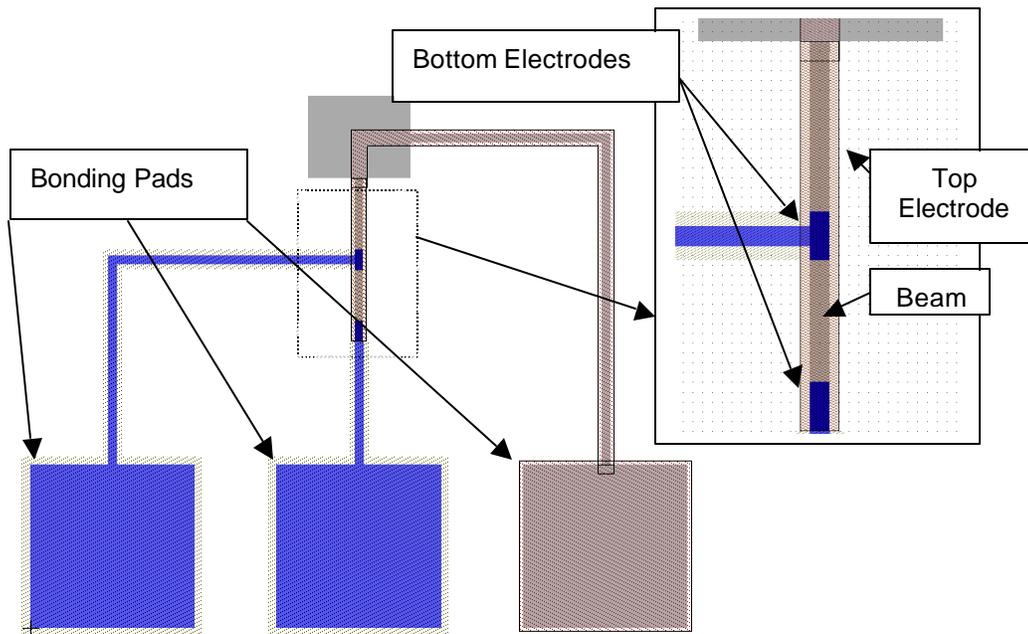
Figure 2-2: Top View (L-Edit Layout) of Cantilever Beam Designed with Micragem
