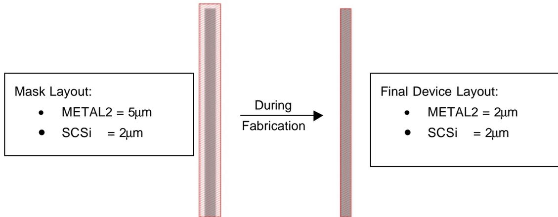
**Figure 3-7: METAL2 Self Aligned to Released Silicon Features**
