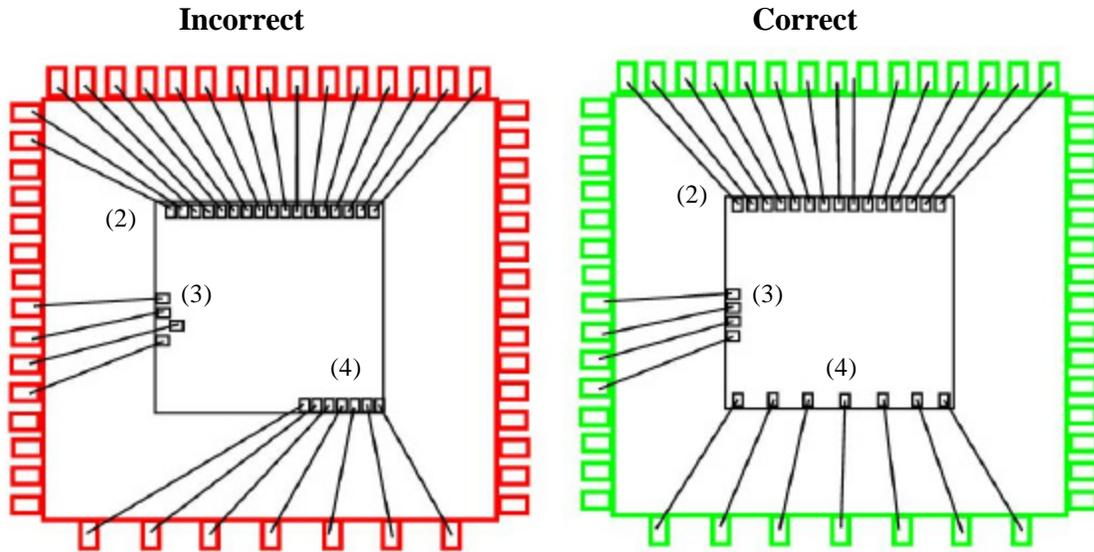
**Figure 5-2: Bonding Requirements Illustrated**
