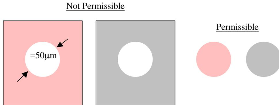
**Figure 3-10: Etched circles less than 50mm not allowed in Metal 2 and SCSi Layers**
