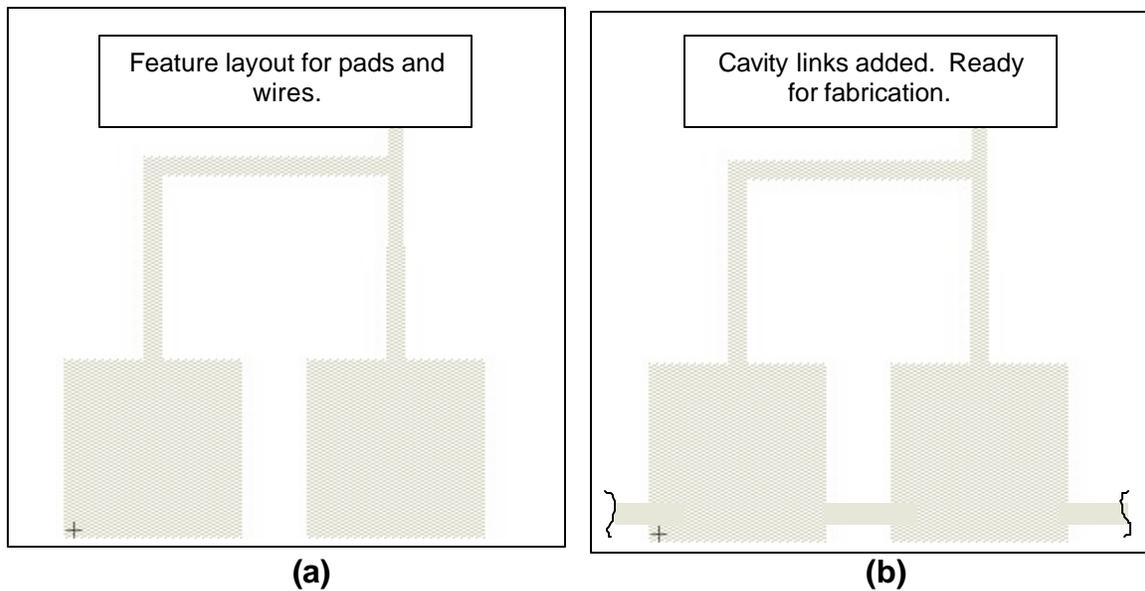
Figure 3-3: PYREX ETCH Layer
