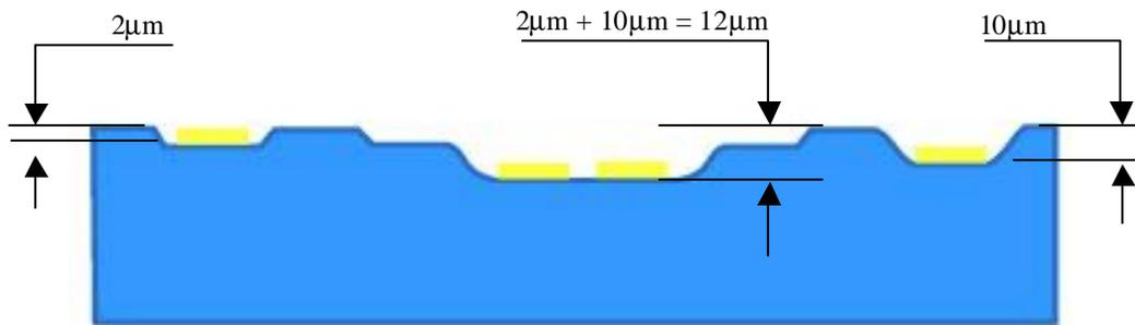
**Figure 3-1: Multi Pyrex Cavity Depths**
