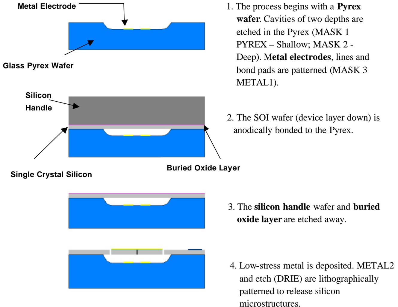
**Figure 1-1: Steps in the Micragem Prototyping Process**
