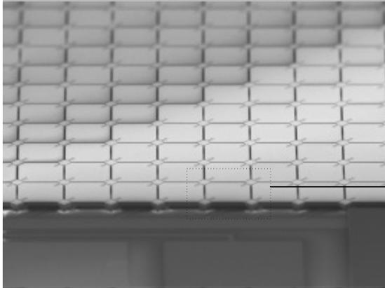
**Example 4: Optical MEMS - Digital Mirror Array**
