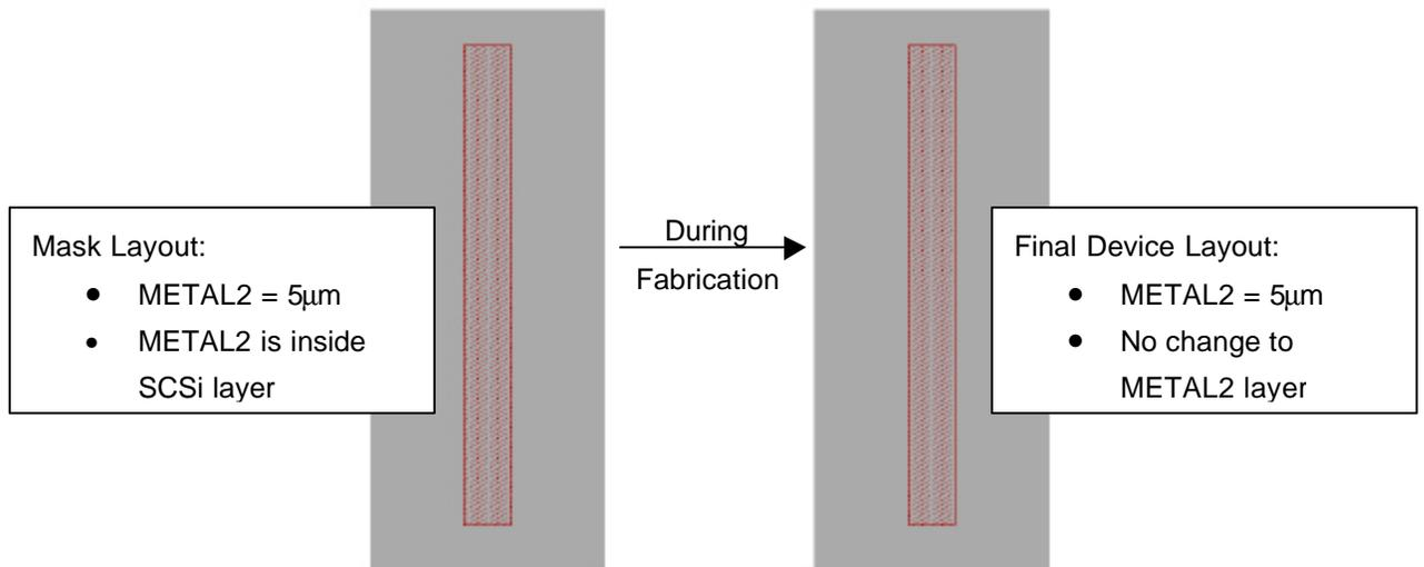
**Figure 3-8: METAL2 is NOT Self-Aligned to SCSi Features Wider than METAL2 Feature**
