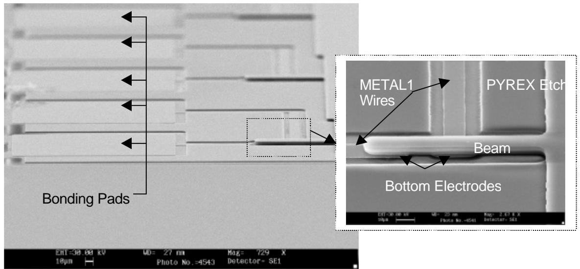
**Figure 2-3: SEM Images of Final Cantilever Device Designed with Micragem**
