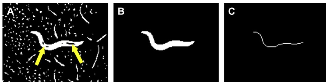
Figure 4. (A) Binarized image with interior holes labeled by arrows. (B) Interior holes filled. (C) Worm skeleton.
