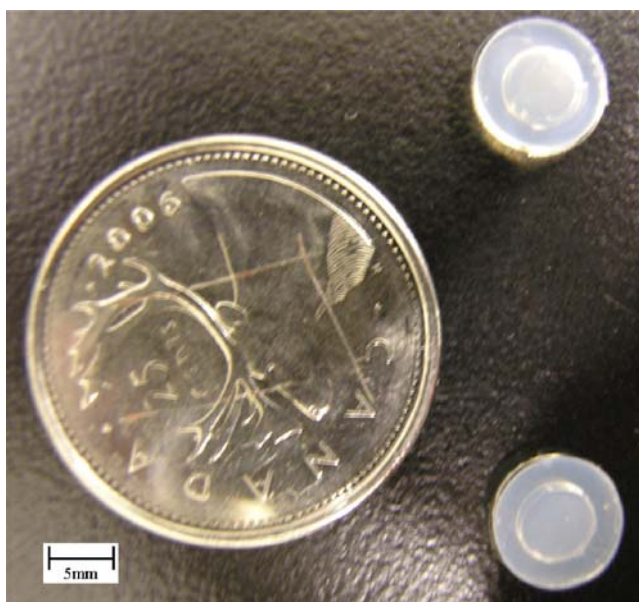
Fig. 6 Prototype microdevices for pH-responsive drug release
