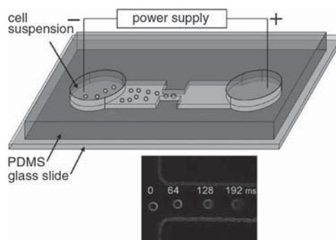
**Figure 5** Electroporation deformation
