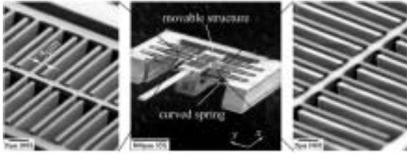
Fig. 3. A cellular force sensor with orthogonal comb drives detailed.
